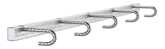
RECOSTAL<sup>®</sup> VHQ are pre-bent reinforcement in a galvanized perforated casing. They ensure quick and safe horizontal continuity of reinforcement between two structural elements of relatively small thickness.
