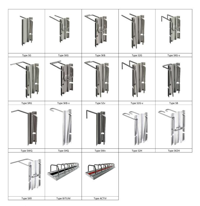
RECOSTAL® RSH Special are pre-bent reinforcement in a galvanized trapezoidal casing compliant with Eurocode 2. They ensure quick and safe horizontal continuity of reinforcement between two structural elements with superior shear force transfer. With a variety of bar shapes in both single and double row arrangements, RECOSTAL® RSH Special are intended to suit any other case that our standard RECOSTAL® RSH, RSV or VHQ cannot cover.
