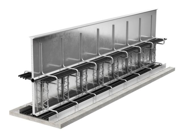
RECOSTAL®DFI-DFA is a permanent formwork made of galvanized metal sheet, bars and additional supports made with lattice girder or bars, allows shoring of expansion joint and internal + external PVC tapes/waterstops installation at the same time. Using this product, concreting on both sides of the structure is possible.
